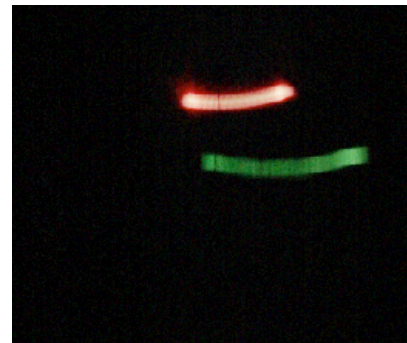
Figure 2 A summary image of a typical video capture, with red (upper line) being the physical pendulum and green (lower line) the simulated image. The image is created by taking the mean color across the video sequence minus the median color across the video sequence, and then normalizing in each color channel.
