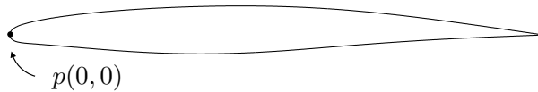
Figure 7: Profile of the BAC3-11 airfoil. Target quantity: pressure p at leading edge, [52, 58].
