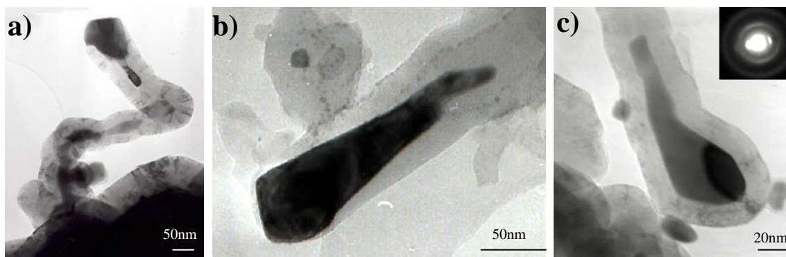
Figures 2a-c. Three varieties of elongated Ni particles characteristic of the nanotube samples (grown at 700°C for 20 min; 600°C for 2hrs; and 700°C for 2 hrs, respectively).
