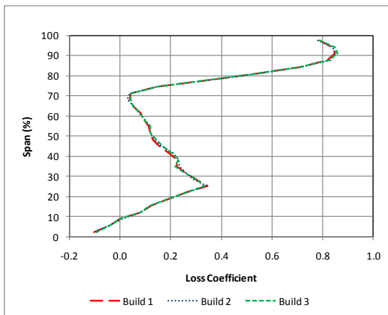
Figure 31: Comparison of span-wise distributions of rotor exit pressure loss coefficient for three builds
