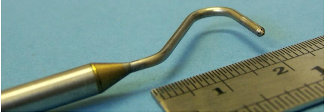
Figure 24: Aeroprobe 5-hole probe
