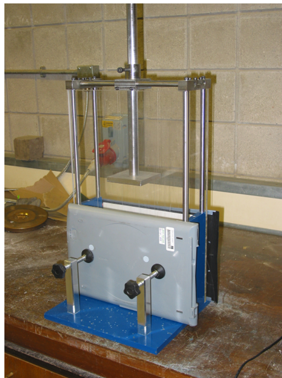
Figure 4.13: Photograph of the compaction chamber with scanner in place. Principal dimensions are shown in Figure 4.12.
