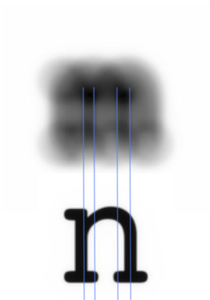
Figure. 8.1: Miss-match in scale of unaberrated 'n' and aberrated 'm' that would not be accounted for by cross-correlation.
