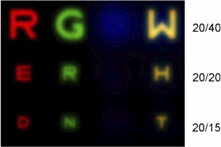
Figure. 4.12: Images (R,G and B) generated with a spectrally weighted polychromatic PSF computed for each phosphor. The linear sum of these (W) gives the correct retinal image accounting for longitudinal chromatic aberration. The faded appearance of B is caused by the luminance scaling of the image (taken from Ravikumar et al. , 2008).
