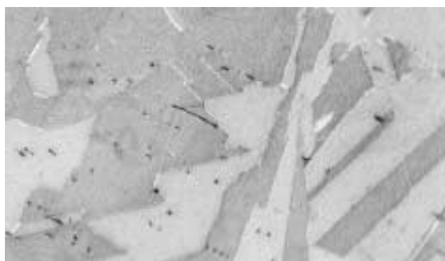
Figure 2: Copper metal etched with alcoholic ferric chloride. Twinned crystals and elongated copper sulphide grains are clearly visible. Optical microscope, magnification 200X. Copper leaf from tomb 393, 3 rd century BC.
