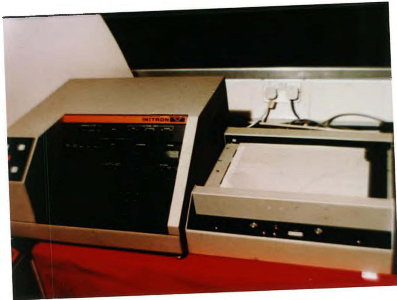
Figure 4.1b Digital control panel and the X-Y recorder.
