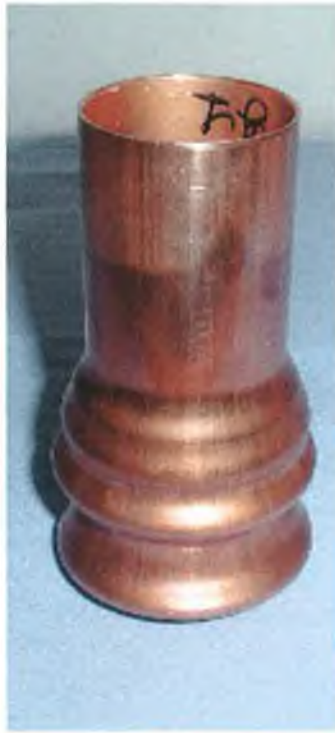
Figure 5.52. : Buckling Failure of a Tube due to High Tube-Rod Friction
