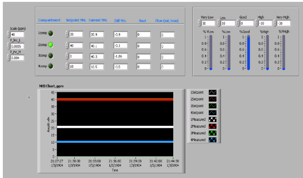
Figure 3.6: User interface of control software. The control software accepts user inputs for all fuzzy parameters and NH 3 setpoints. Real-time graphs and readings of the current NH 3 concentration, signal voltage and volumetric flow rate of all four compartments are displayed.
