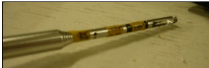
Figure B.7: Pre-labeled distances on hot-wire anemometer probe. A velocity profile could be quickly constructed by recording the velocity measured inside the pipe at each pre-labeled distance.
