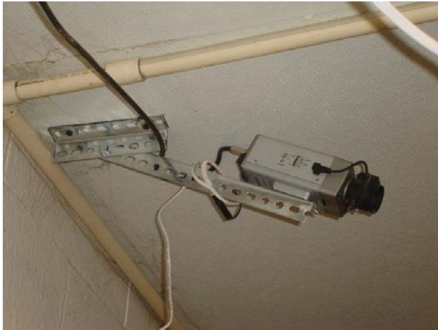
Camera mounted at ceiling to record three gilts in one temperature/lighting treatment
