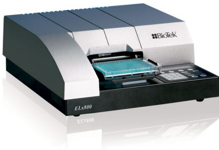
Example of BioTek plate reader used in lymphocyte proliferation assays; This image is property of BioTek Instruments, Inc. ( www.biotek.com )
