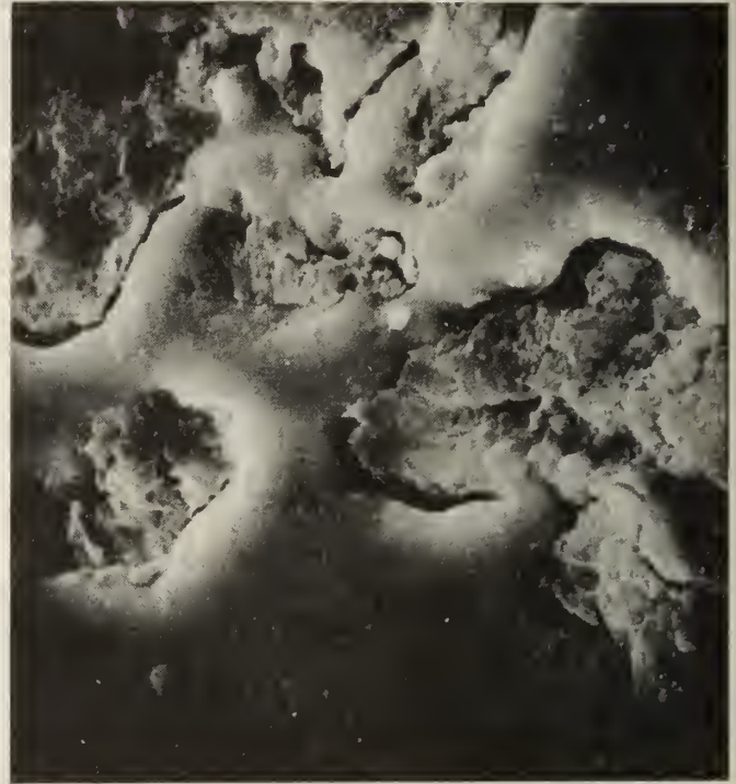
Figure 25 Particle with clay matrix and quartz and barite inclusions. 2130X
