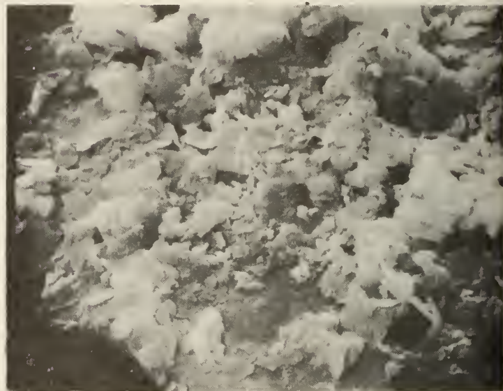
Figure 10. Illite from liquefaction residue. 10,413X
