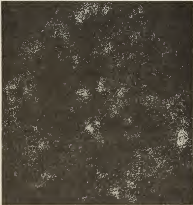
Figure 24 X-ray map of sulfur for Figure 21. 1105X
