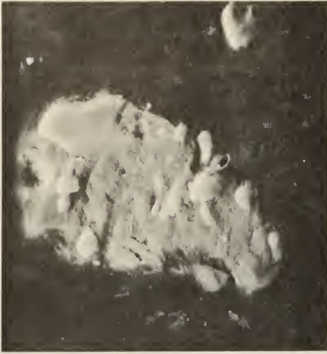
Figure 25 Particle with clay matrix and quartz and barite inclusions. 2130X
