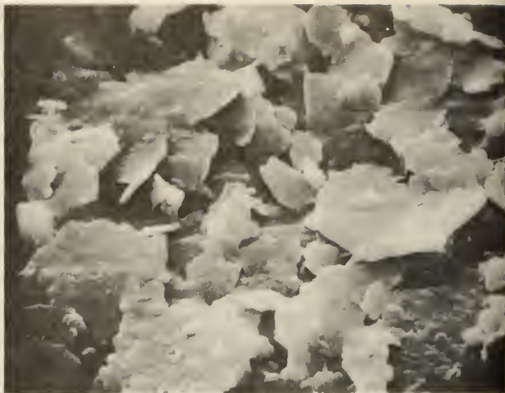
Figure 9. Kaolinite and other clay minerals from liquefaction residue. 5253X
