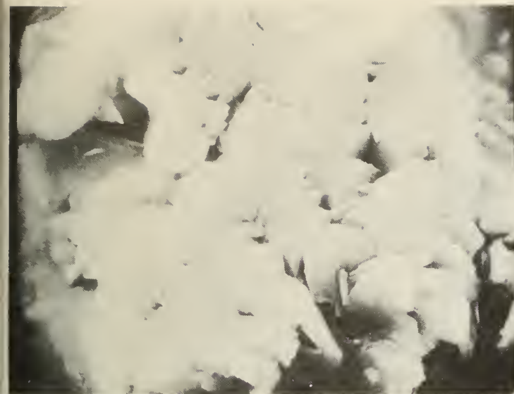
Figure 11. Euhedral kaolinite from liquefaction residue. 2491X
