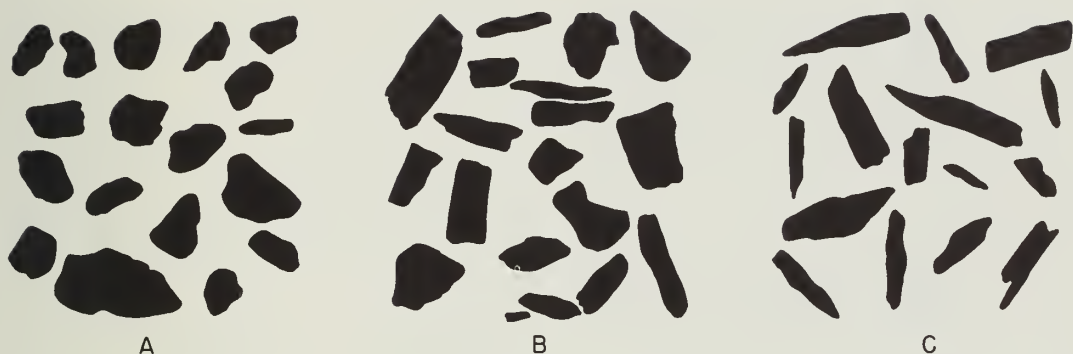
Fig. 7 - Shapes of shale fragments in well cuttings: A - Caseyville, B - Chester, C - Selected lath-shaped Chester.
