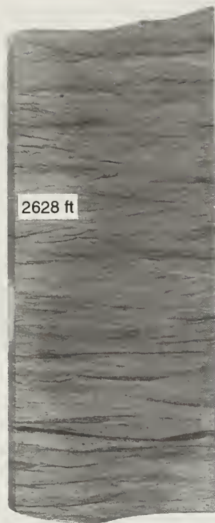
Figure 16 Ripple-laminated, extremely fine-grained, green sandstone and siltstone facies underlying the reservoir cross-bedded sandbar facies through much of Zeigler Field (sample from the Gallagher Drilling Company no. 2 Mack at 2,628 ft).
