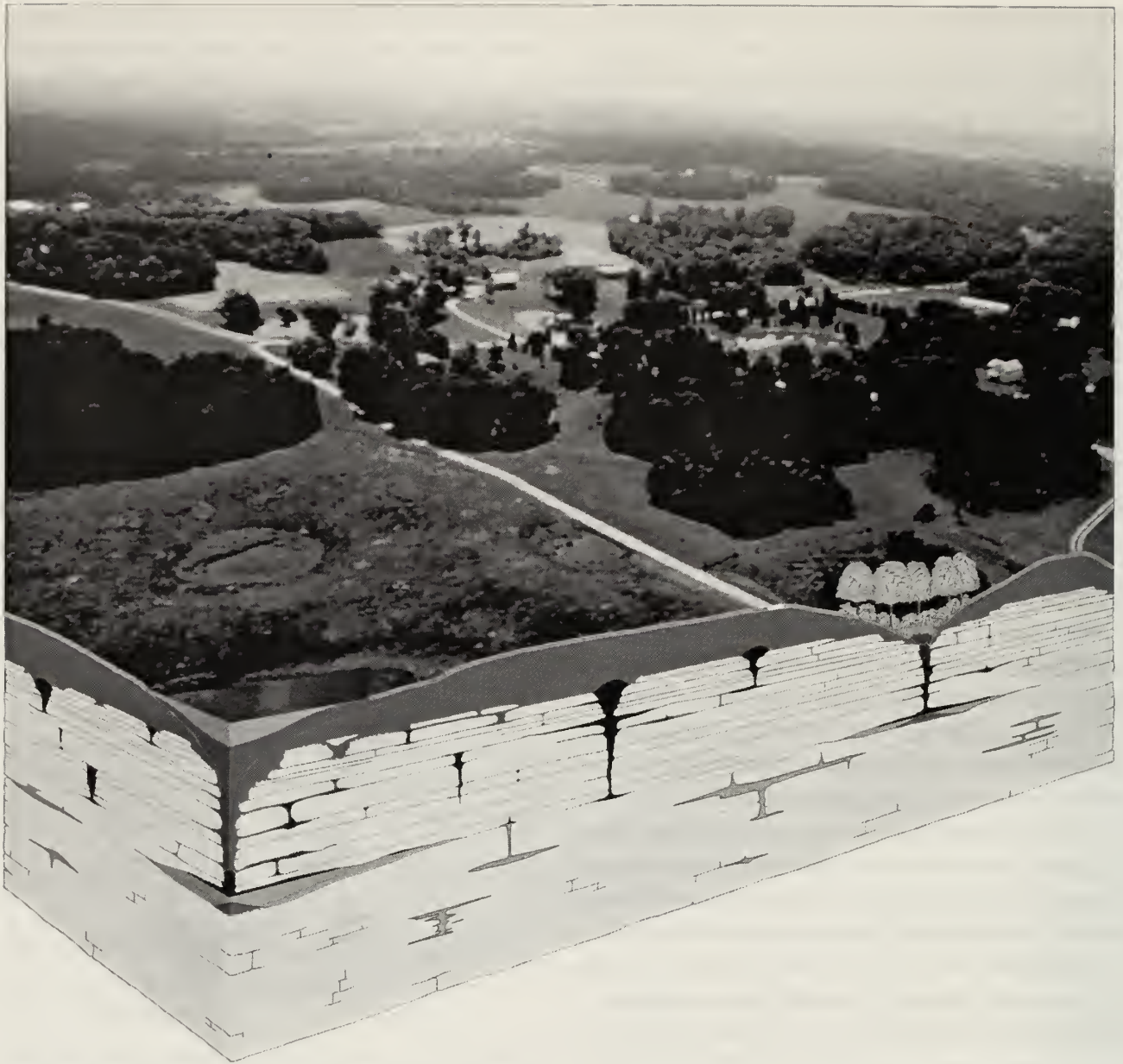
Figure 2. A block diagram of the karst terrain of the sinkhole plain showing bedrock and the relationship between crevices and sinkholes. Notice that the bedrock dissolves along bedding planes forming horizontal opening that can extend, as conduits, for miles. If accessible, these conduits are referred to as caves.
