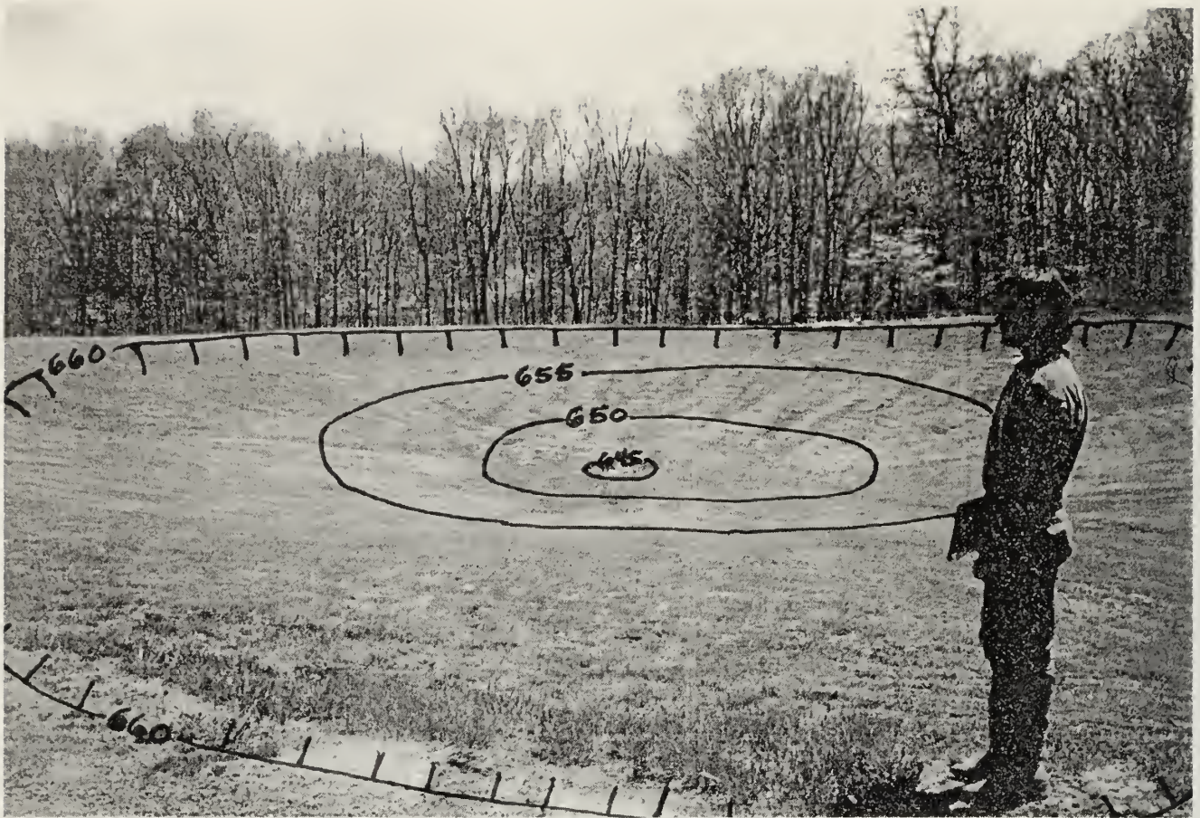
A circular sinkhole in the sinkhole plain with contours superimposed on the photograph. Contour interval is 5 feet. The sinkhole was 85 feet in diameter and led to a 5 foot deep depression in the center that acted as the drain to a bedrock fissure. Any runoff from rain that falls within the hachured contour will flow toward the center of the sinkhole and into the bedrock fissure.
