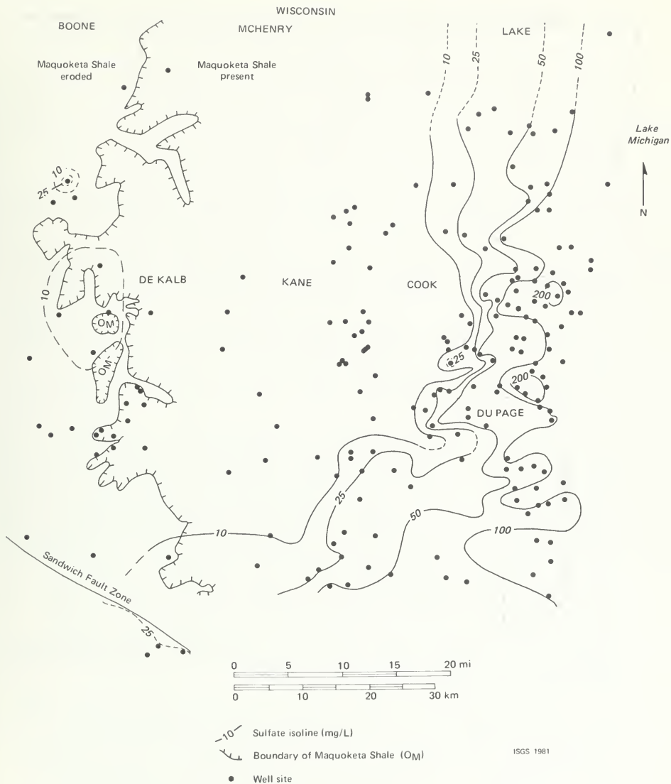
FIGURE 4. Distribution of dissolved sulfate in groundwater of the Cambrian-Ordovician aquifer system for a region of northeastern Illinois. (From Gilkeson and Cartwright, in press.)
