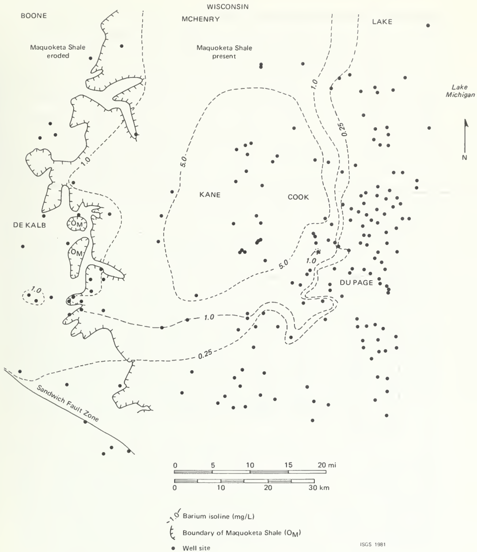
FIGURE 5. Distribution of dissolved barium in groundwater of the Cambrian-Ordovician aquifer system for a region of northeastern Illinois. (From Gilkeson and Cartwright, in press.)
