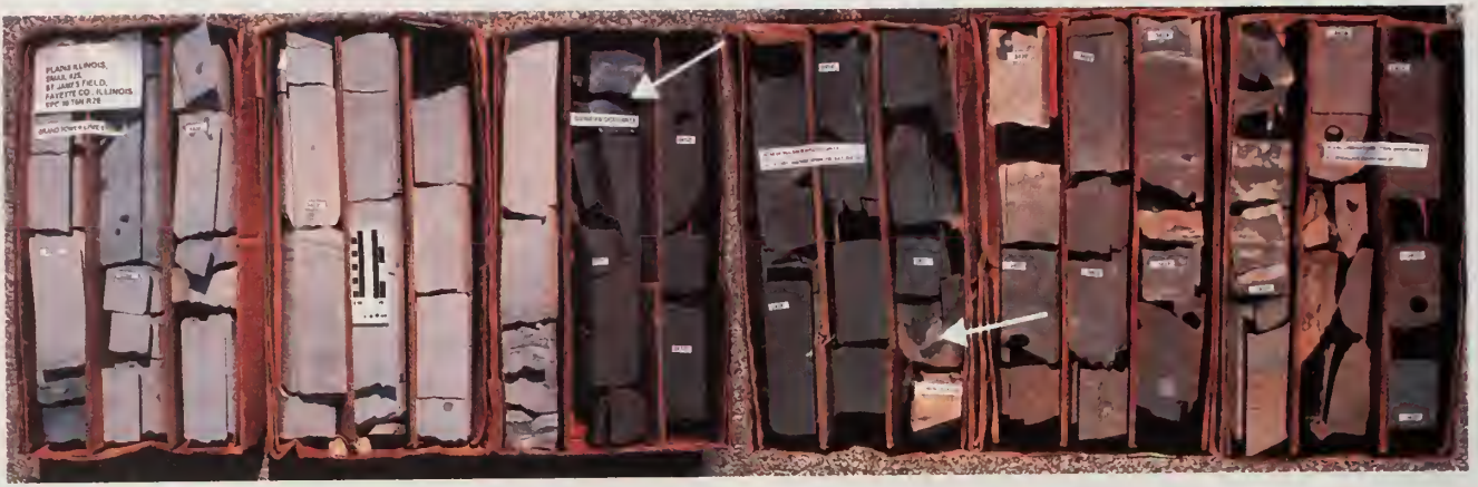
Figure 31 Core from the Plains, Illinois, Small No. 25 in the St. James Field, Sec. 36, T6N, R2E, Fayette County. This is well No. 1 in cross section C-C'. The cored interval is from the Middle Devonian Grand Tower Limestone through a cherty zone in the Geneva Dolomite. The upper contact (at arrow) of the Geneva Dolomite with the overlying Grand Tower Limestone is abrupt. There is no transition zone from the bioclastic grainstone above and the brown Geneva Dolomite below. The contact between the Geneva Dolomite of the typical brown sucrosic dolomite with the underlying cherty interval also is abrupt (arrow).
