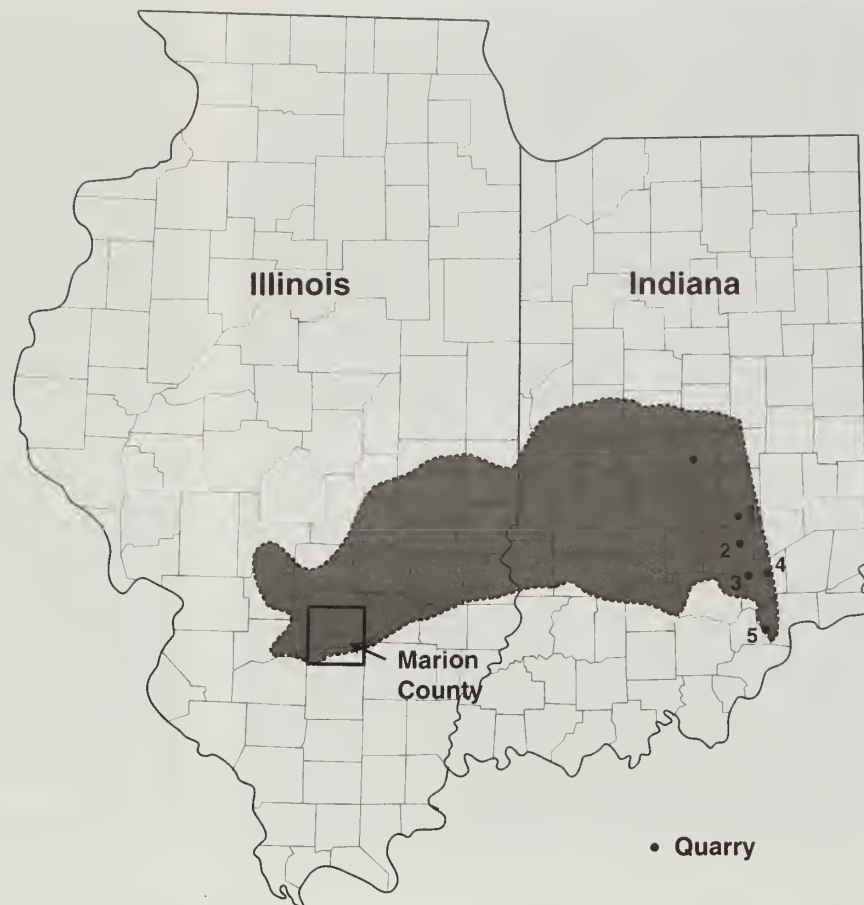
Figure 8 Distribution of the Geneva Dolomite in Illinois and Indiana. The Geneva reaches a maximum thickness of about 90 feet in east-central Illinois; thins to zero in southern Marion County, Illinois; and outcrops in a series of quarries (numbered 1 through 5) in southeastern Indiana, where it is 20 to 30 feet thick. (Modified from Perkins 1963, Schwalb 1955.)
