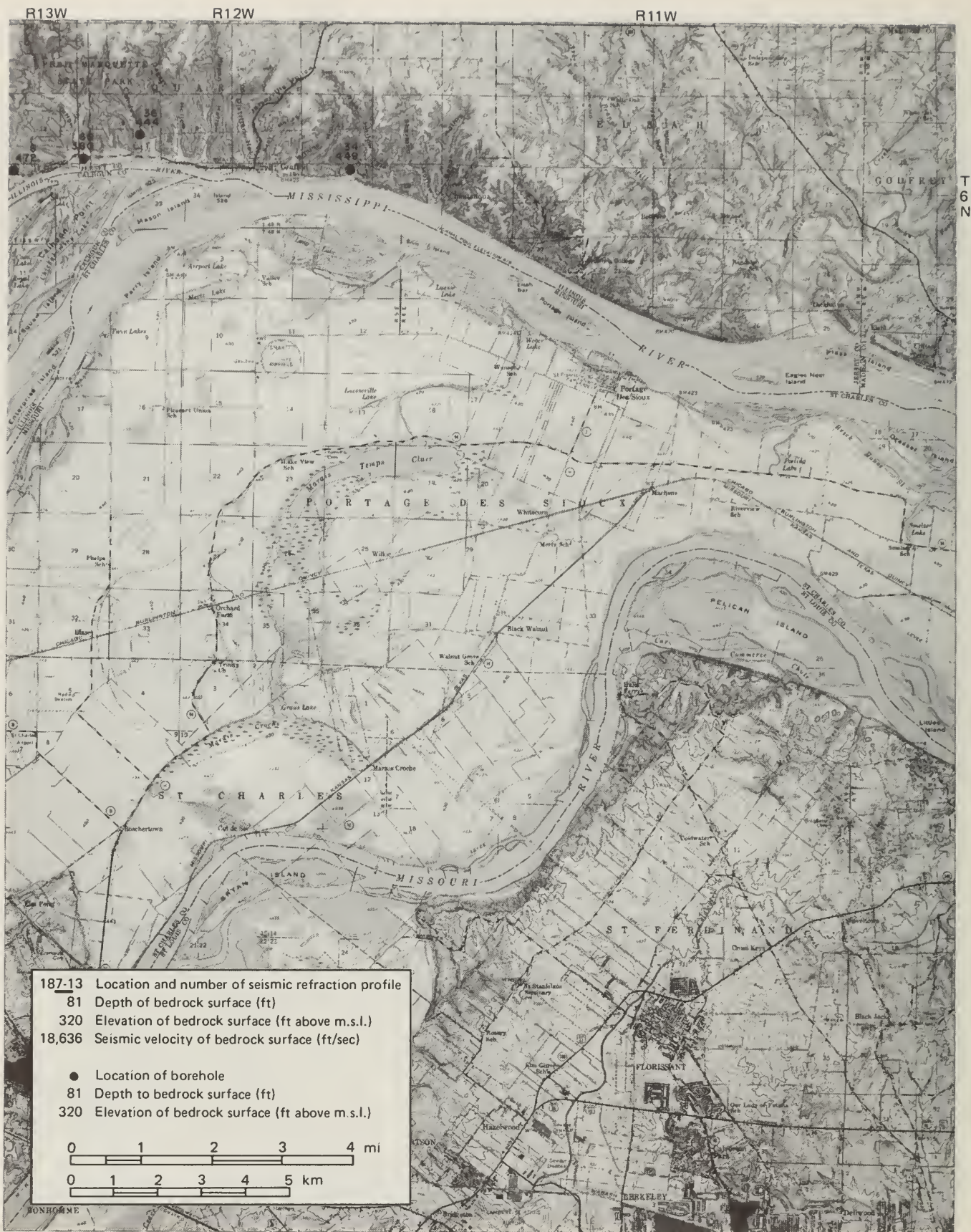
Figure 4g. Seismic refraction data and borehole data for the St. Charles 15-minute quadrangle.
