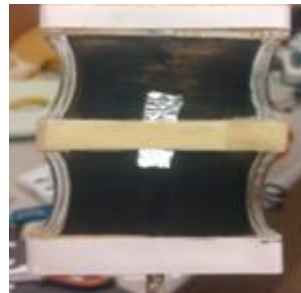
(b) Ball joint actuator module connected to testing setup
