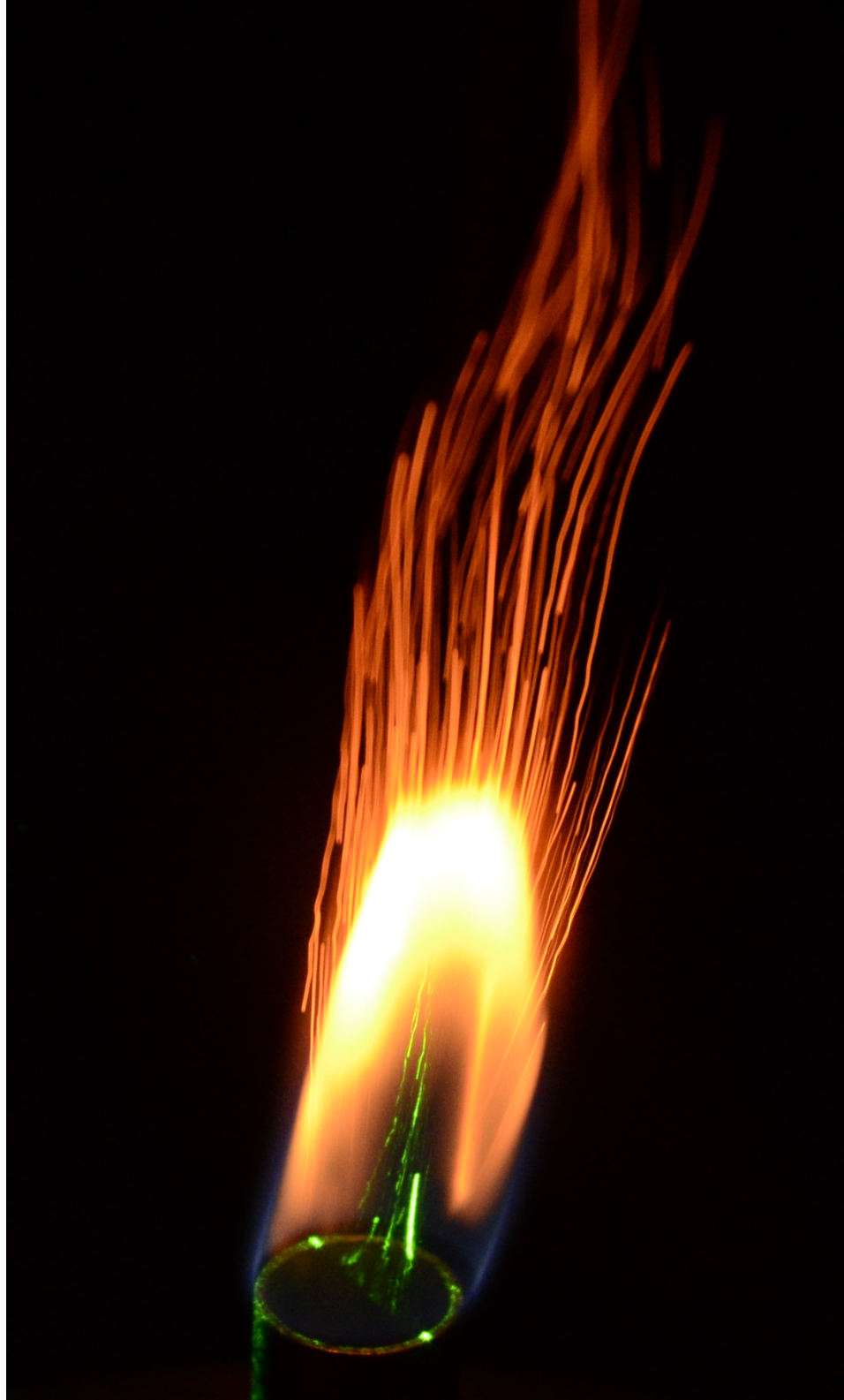
Figure B.2: Coal particles interacting with the flame front. (Captured at a 45° angle to the laser sheet).
