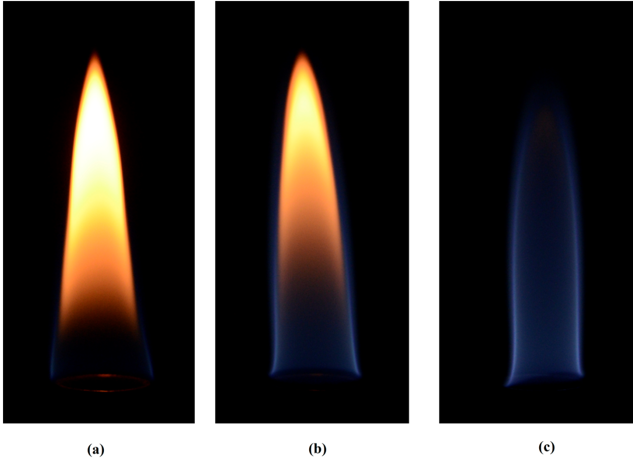
Figure 3.12: (a) Non-diluted \text{CH}_4 diffusion flame (b) Weakly diluted \text{CH}_4 diffusion flame (c) Strongly diluted \text{CH}_4 diffusion flame strongly diluted with \text{N}_2 . No laser sheet present.
