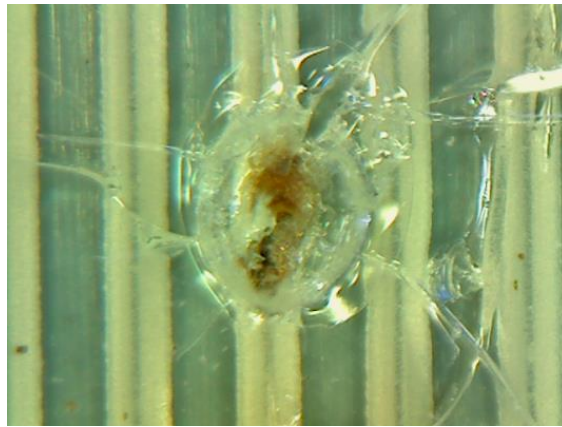
Figure 4.2. Optical microscope image of failed glass-alumina device
