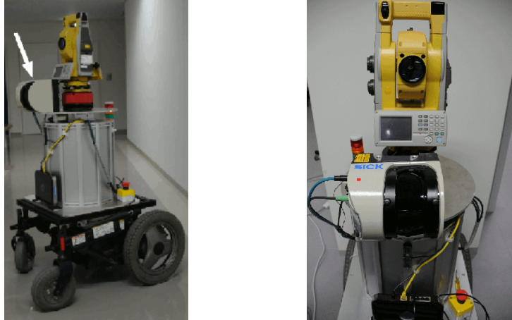
Figure 2: The left picture shows the robot used in our experiments. A white arrow indicates the laser range finder used to take scans. The right picture presents a closer look at the laser range finder.
