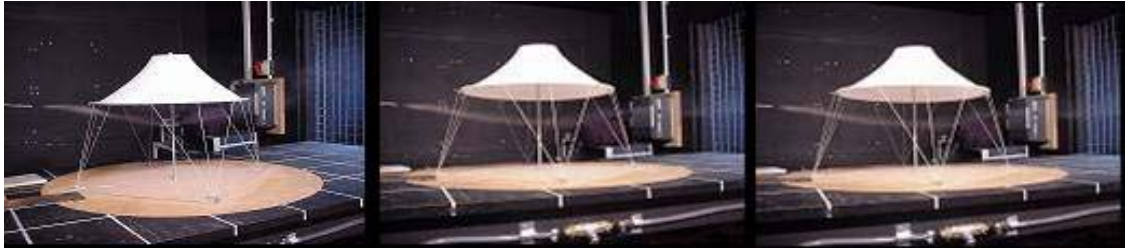
Figure 5. Wind tunnel experiment showing the effect on airflow of a conical membrane with closed apex
