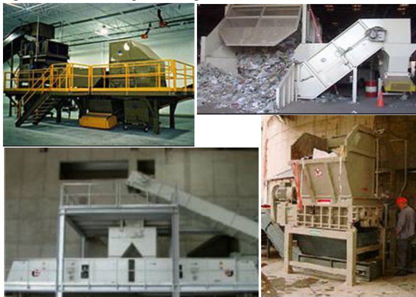
Figure 6: Removing metals for further use; Machine for non-ferrous metals removal; Removal of heavy materials; Shredding to smaller size
