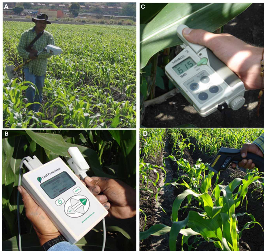
FIGURE 4 | Different devices to evaluate plant growth, phenology and water status. (A) spectroradiometer with active sensor to measure the normalized difference vegetation index (NDVI); (B) porometer to measure stomatal conductance; (C) leaf chlorophyll meter; (D) infrared thermometer to measure leaf temperature.
