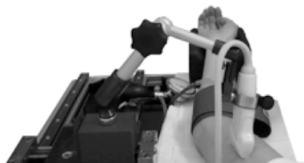
Fig. (3). Assessment of brachial artery flow mediated dilation (FMD). Right panel shows the stereotactic clamp to hold the probe and to adjust the images by means of micrometric screws. Graphs on the left panel show changes in diameter ( d , bottom) and shear stress ( SS , top) obtained by real-time analysis of B-mode and doppler signal during FMD assessment. Timing of cuff inflating and deflating for inducing and stopping forearm ischemia are also shown in the cartoon.
