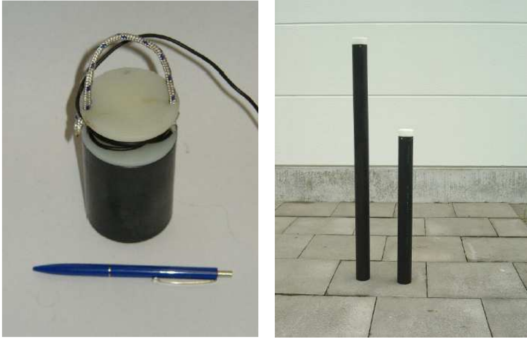
FIGURE 2.6: Electrode EFP-06 employed for electric field measurement (left panel). Magnetometers MFS-06 (left) and MFS-07 (right) (right panel).
