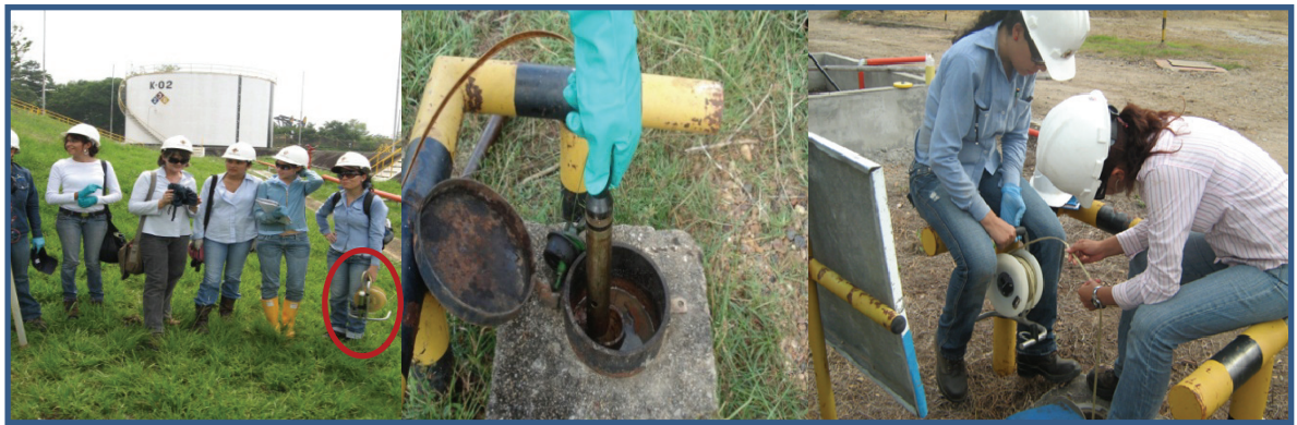
Figure 13. Measurement of the static levels in field
