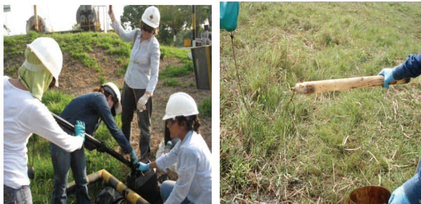
Figure 15. Oil recovers and measurement of water conductivity into control wells
