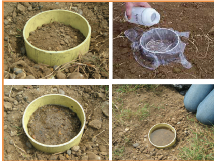
Figure 10. Measurement of soil infiltration in situ
