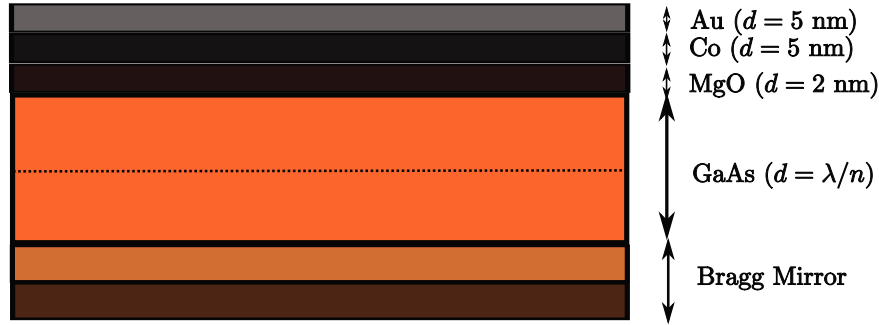
Figure 4.4: Modeled spin-structure shown schematically including the gold electrode (Au), magneto-optical spin-injection layer (Co), tunnel barrier (MgO), active layer GaAs with active plane in the center and Bragg structure.
