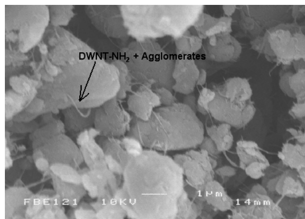
Figure 2. Amino-modified double wall CNTs in "as received form"
