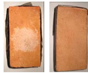
Fig. 11 Efflorescence test results
