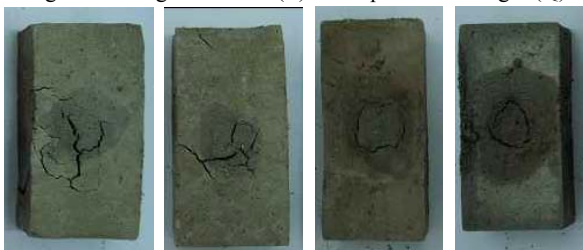
Non-baked specimens: severely damaged during tests
