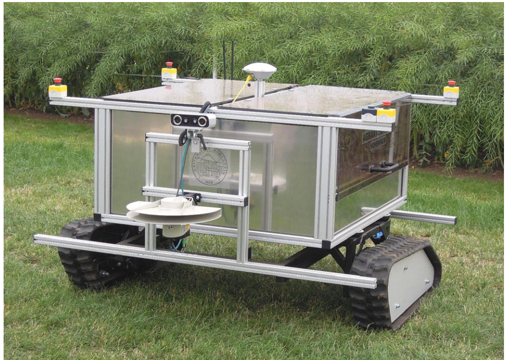
Fig. 2 Electric powered autonomous tractor with GNSS based navigation for sensing (scouting and monitoring)
