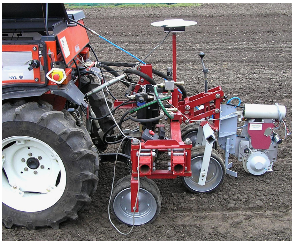
Fig. 4 Autonomous tractor with GNSS based navigation and side-shift frame for highly accurate placement of seeds (punch planter)
