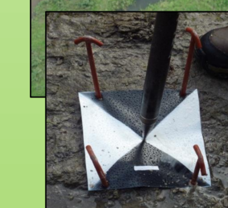
Figure 6. An artificial ground control point (GCP)
