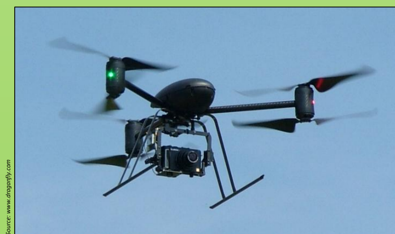
Figure 2. The Draganflyer X6 – an unmanned aerial system
