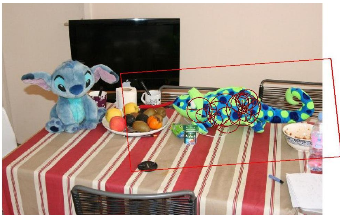
Figure 4.1 The circles in the images indicate the SIFT features used to identify the presence of the target object. The outer parallelogram shows the boundary of the target image under the affine transform used for recognition.
