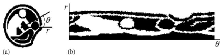
Figure 1.8 (a) An original shape in polar space; (b) polar-raster sampled image plotted in Cartesian space [20]
