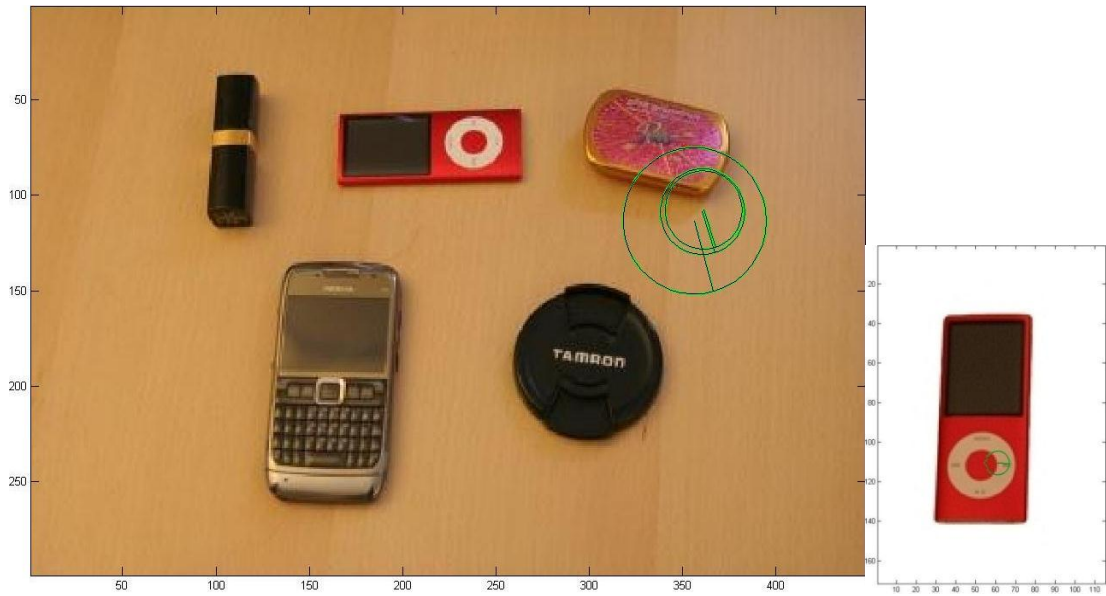
Figure 4.3 In the left image, clustered SIFT shape features have been located, with their correspondences on the prototype object marked in the right image.
