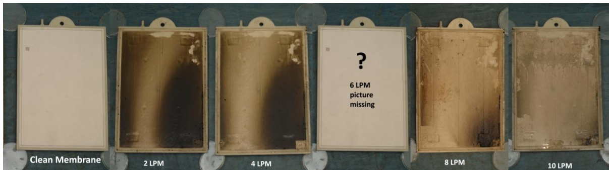
Figure 4-9 Membrane pictures during operation with re-increasing the gassing rate
