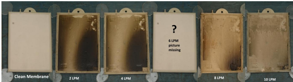
Figure 5-6 Membrane pictures as the gassing rate was increased.
