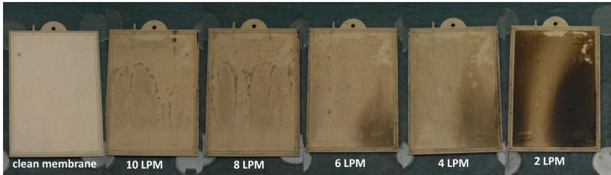
Figure 4-8 Membrane pictures during operation with decreasing gassing rate
