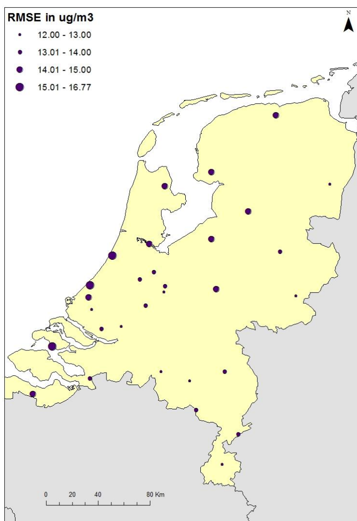
Figure 7.7 Proportional circles of the residual error (RMSE) at each monitoring sites
