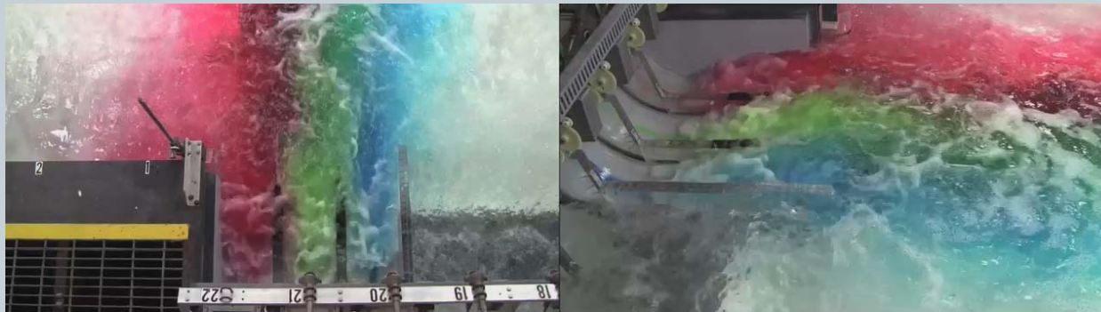
Hydraulic jump reaches face of spillway with forebay elevation of 488.0 ft and river flow of 414,900 cfs
