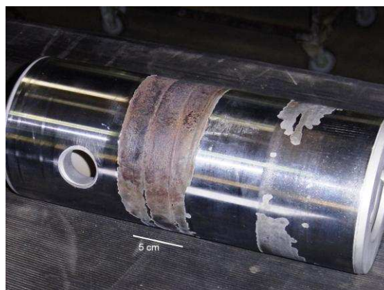
Figure 3. Typical landing gear component exhibiting chrome plate damage
