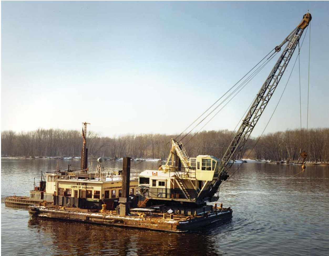
Dredging the Mississippi River: The Dredge Hauser, a small dredge operated by the St. Paul District. (Photo courtesy of St. Paul District, Corps of Engineers)
