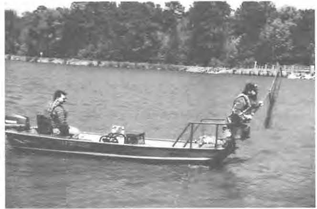
Fig. 3.1. Jon-boat showing positioning of night-lighting equipment (bow rails, lights, converter box, and generator) and personnel. From King et al. (1994).
