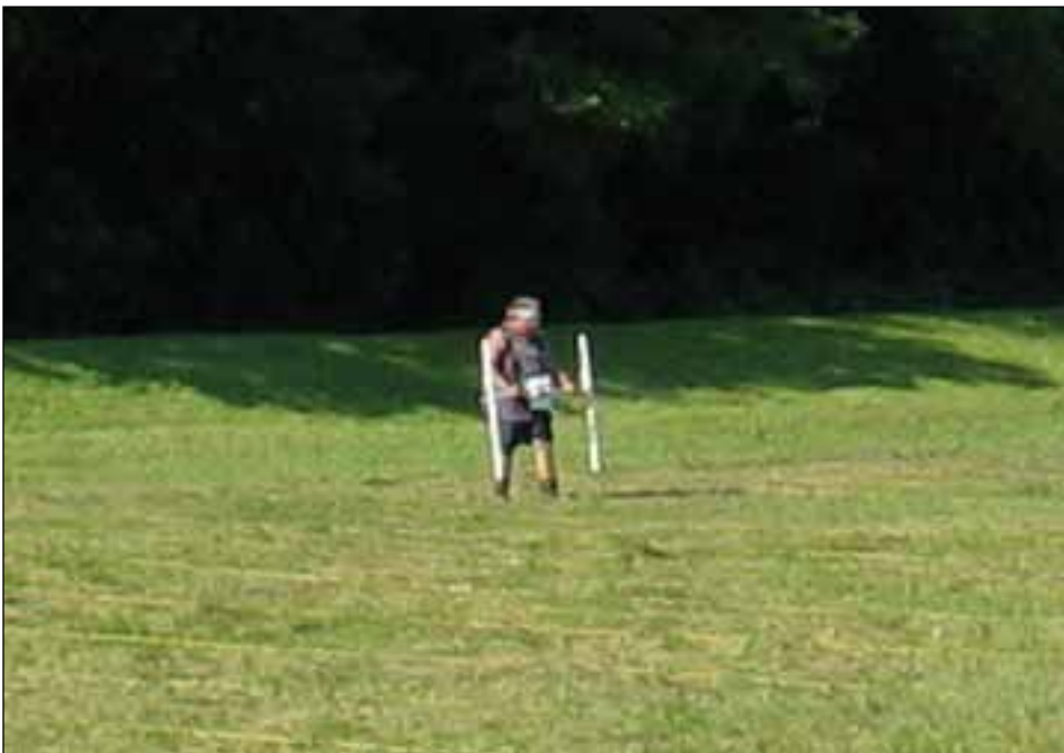
Figure 6. Conducting magnetic survey with dual fluxgate gradiometer.
