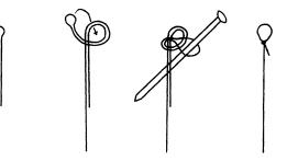
Fig. 1. Tie a single loop at one end of the mono-filament line, leaving a small tab (3-5 mm) at the base of the single loop.
