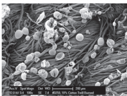
Figure 8. SEM micrographs of different regions of fabric: (1) print cloth (2) twill fabric with.
