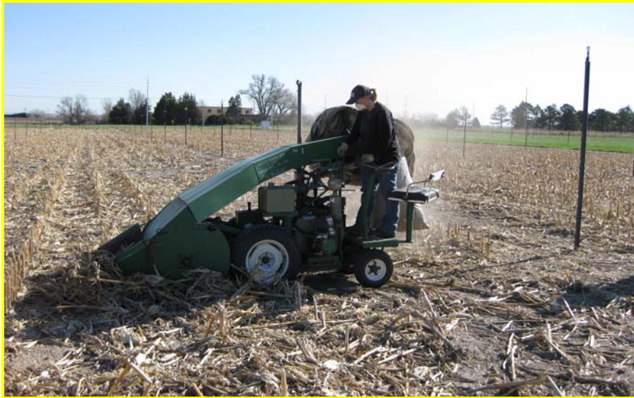
Figure 1. Removing crop residue to create four bare-soil plots using a flail chopper, April 2009. After the flail chopper, additional residue was removed by hand-raking and shoveling. Residue was removed from the same four plots in April 2007 and 2008 using similar methods.
