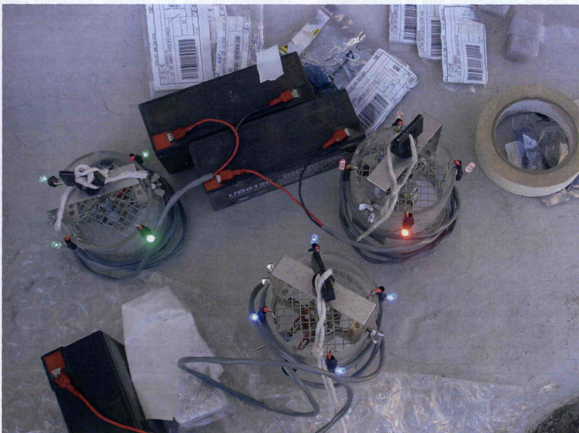
Figure 1. Light-emitting diode (LED)-modified CDC light traps (model 512, JW Hock Company, Gainesville, FL). Traps were designed to accommodate plug-in type LEDs to facilitate quick replacement or color change.
