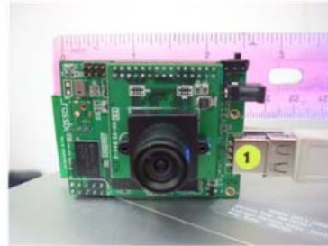
Figure 1. CITRIC camera: the wireless embedded smart camera platform employed in the experiments.
