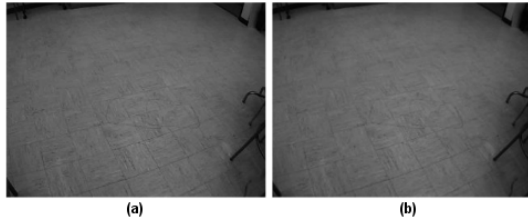
Figure 5. QVGA images captured by (a) using the API software library down-sampling subroutines and (b) performing hardware-level down-sampling on the micro-controller of the OV9655.
