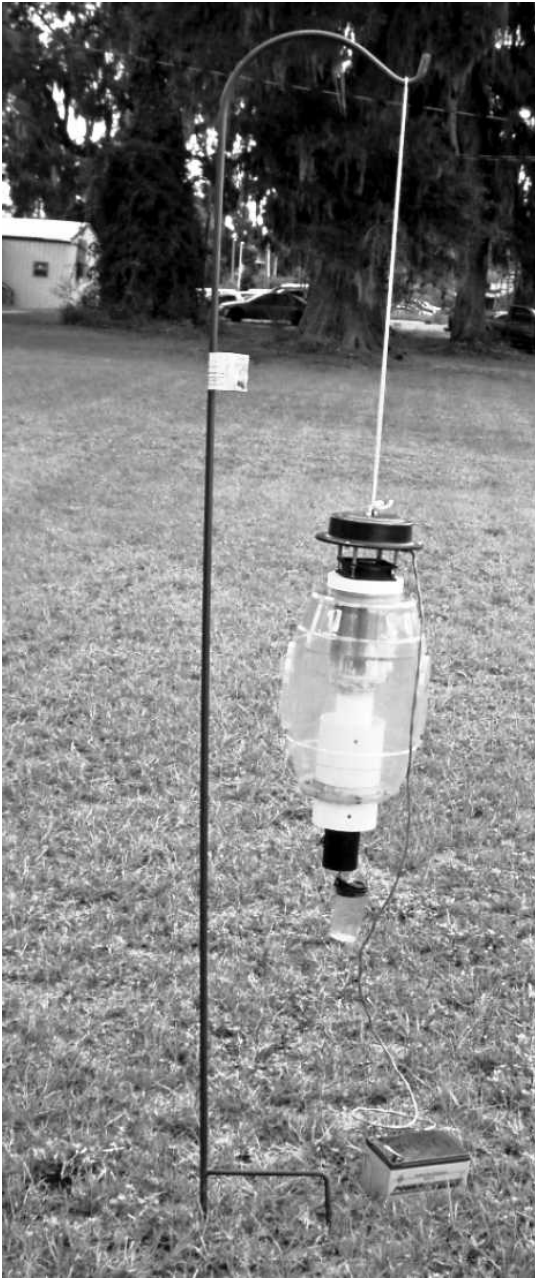
Fig. 1. Mosquito Magnet™-Experimental trap with jar of blend suspended near the carbon dioxide outlet port.
