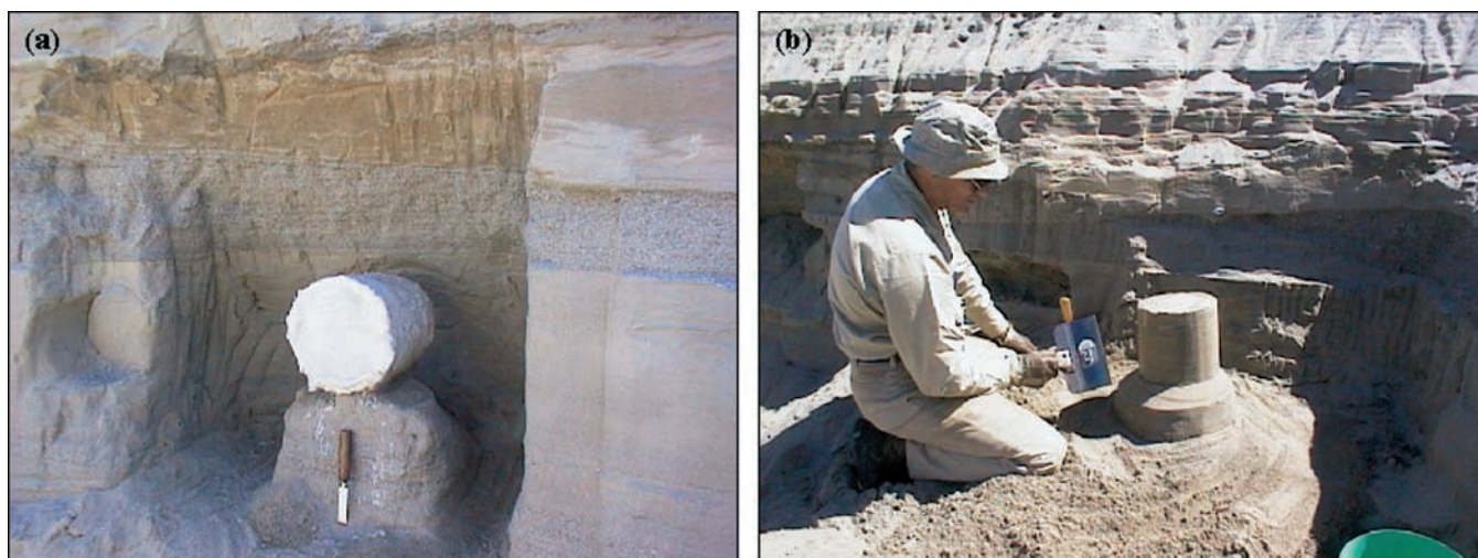
Fig. 3. Harvesting of undisturbed cores from the Hanford Formation. (a) Paraffin wax-coated horizontal core, and (b) sculpting of vertical core.
