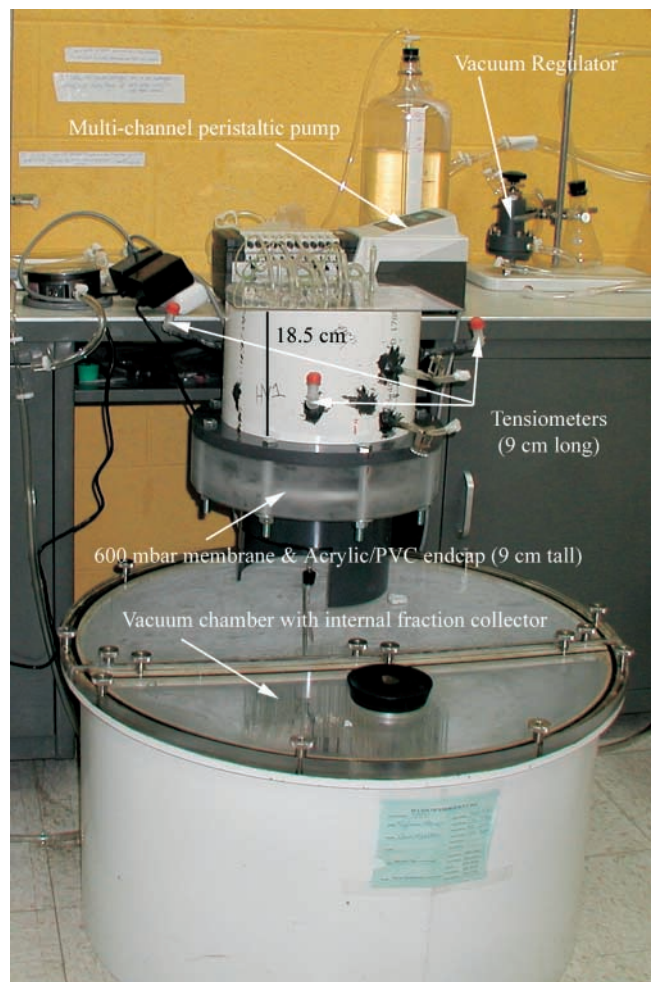
Fig. 4. Experimental apparatus for conducting unsaturated flow experiments in undisturbed cores.
