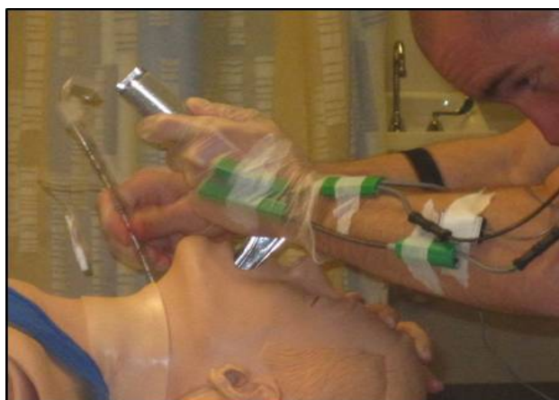
Figure 6 – Location of goniometer and torsionmeter sensors on left hand and arm
