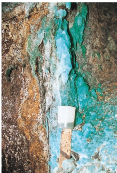
FIG. 4. Growth of cuprian melanterite in a manway of the Richmond Mine with stalactite dripping pH = -0.7 water into plastic beaker. (Photo by D.K.N. and C.N.A.)
